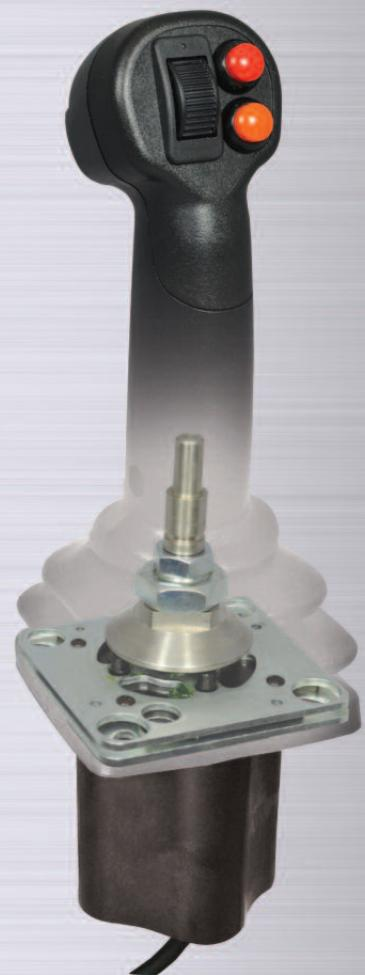
\*JH Joystick shown with small universal grip incorporating Hall Effect Pushbutton Switches (HP7's) and a Hall Effect Thumbwheel Switch (HTW).
